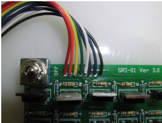
Cable wiring for the OWI-535 Robotic Arm, see text.
