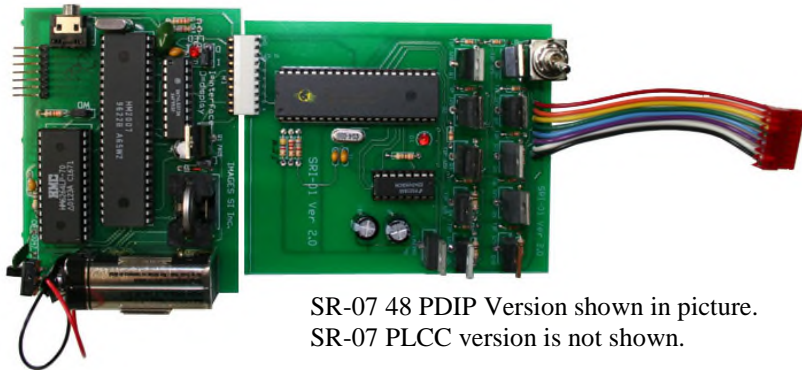
Figure 3 Top view of SR-07 and speech interface board
